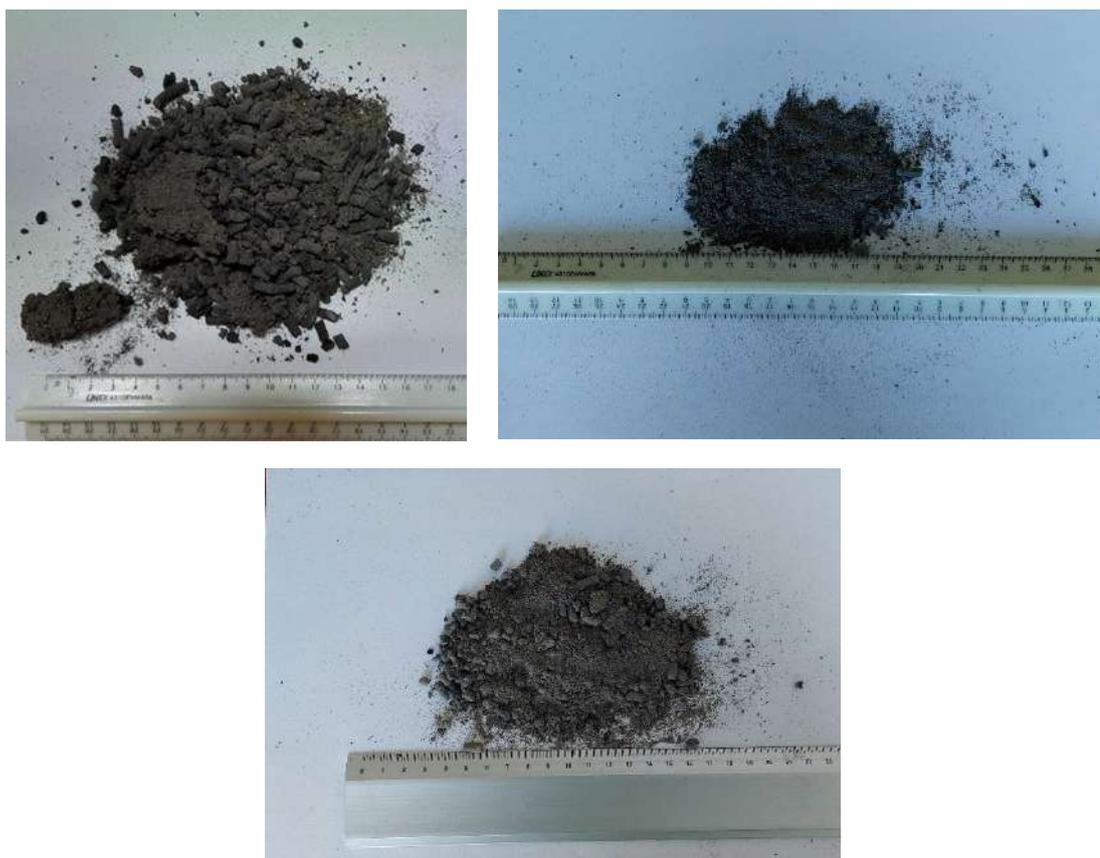
Figure 29. Ash samples from: (top left) wood pellets, (top right) urban prunings with coffee residues (CU10), (bottom) sawmill residues with coffee residues (CS10)
