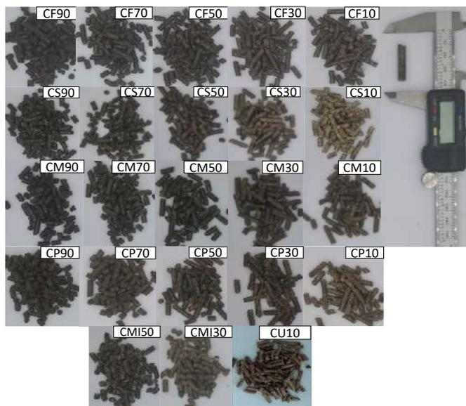
Figure 23. Mixed coffee pellets produced at ESEK plant
