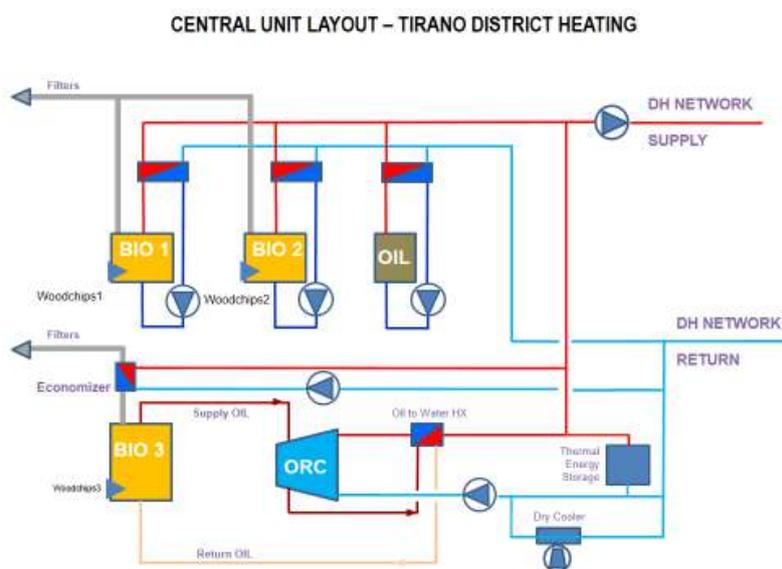
Figure 11. Tirano district heating central unit layout
