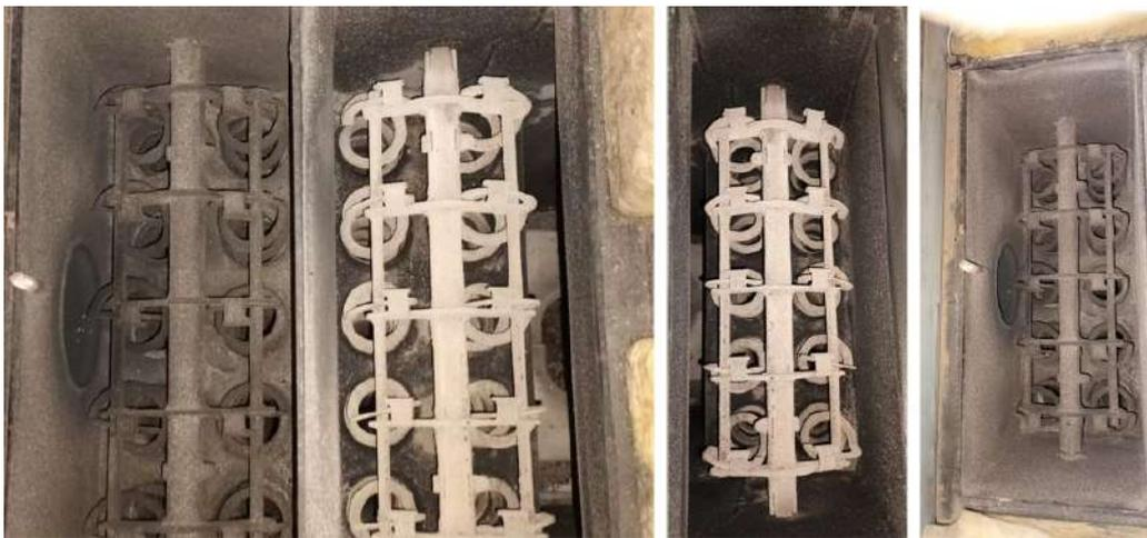
*Figure 5. Images of the heat exchanger of the biomass boiler after the test.*
