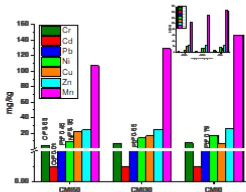
Figure 47. Minor (down) elements (mg/kg d.b.) of coffee pellets mixed with miscanthus
