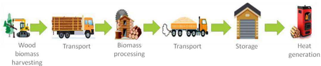
*Figure 12 Diagram of value chain operations (forestry biomass)*
