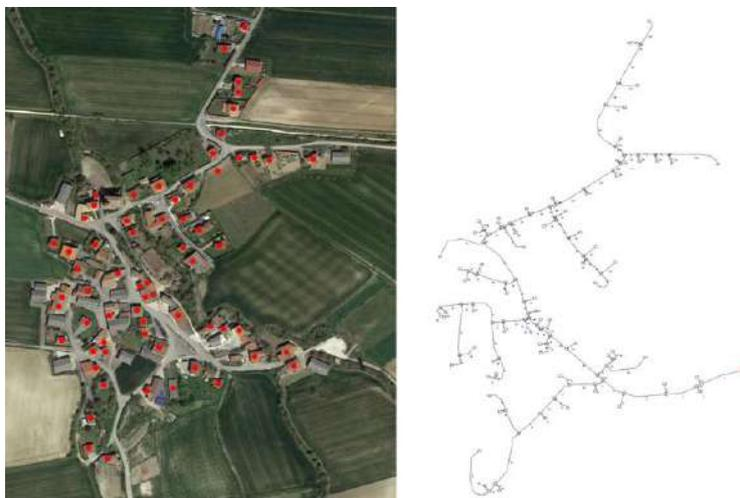
Figure 7 Consumption points (houses, right) and distribution of the network (left) along Aberasturi.
