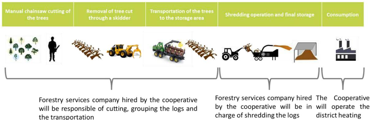
Figure 1 Diagram of value chain operations (forest residues)
