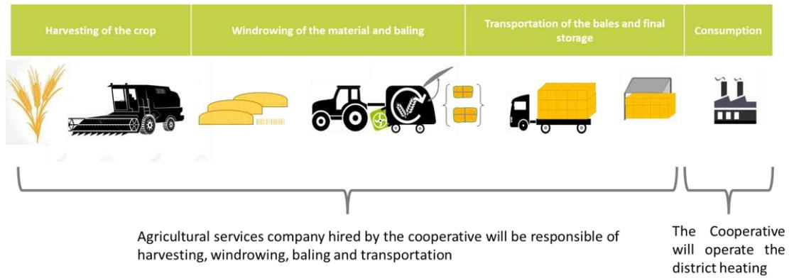
Figure 2 Diagram of value chain operations (herbaceous biomass)
