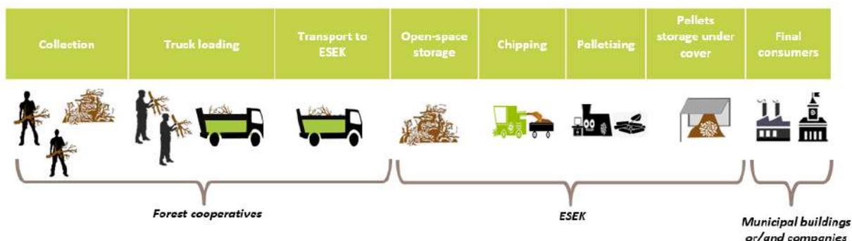
Figure 36 Diagram of value chain operations (forest residues)
