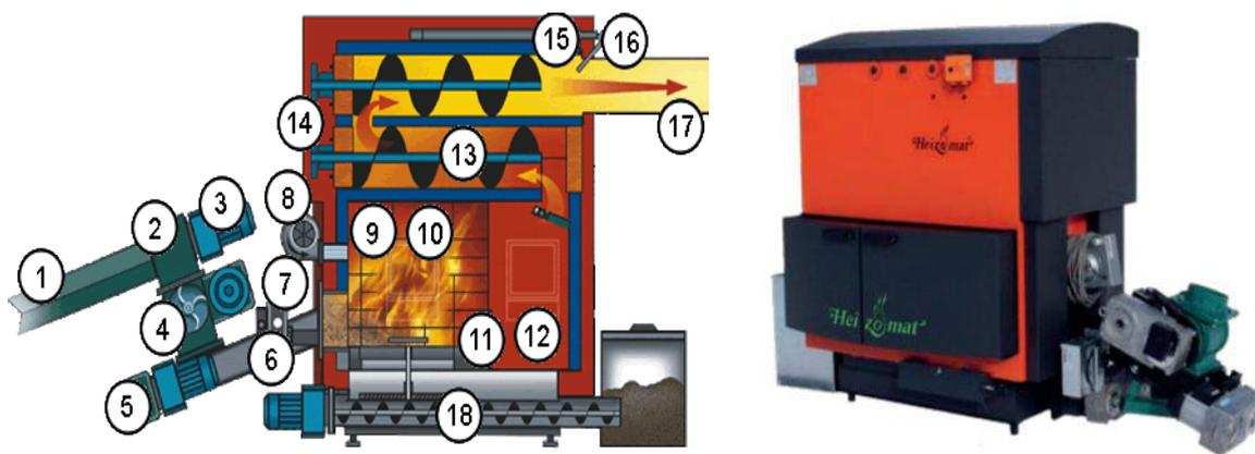
Figure 29. RH-AK 30-990 kW Wood Chip Boiler Cross Section [11]:
