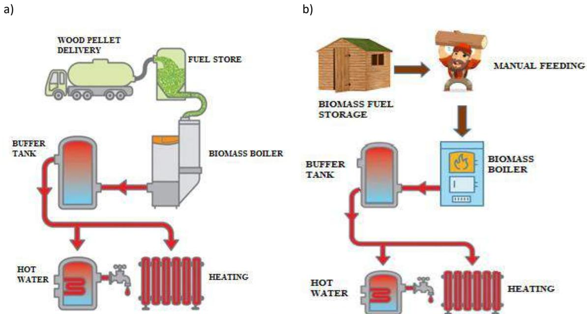
Figure 2. Main components of typical biomass direct heating installations [5]: a) automatic system of direct heating; b) manual system of direct heating.
