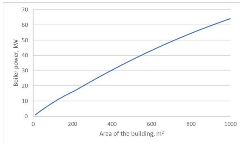
Figure 5. Thermal power of the boiler vs. Heated surface area of the building (in a temperate climate) [21].
