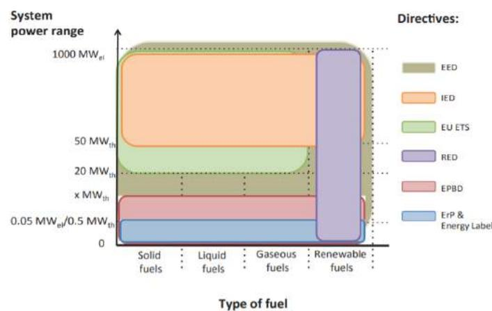
Figure 71: EU policies relevant for CHP based on fuel type and nominal power range [42]
