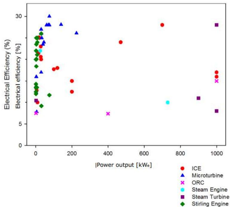
Figure 17. Electrical efficiencies of biomass conversion technologies based on power output [58].
