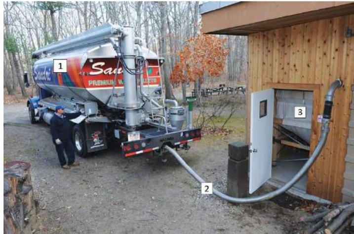
*Figure 32. Pellets delivery process with the use of a tanker [14]:*
