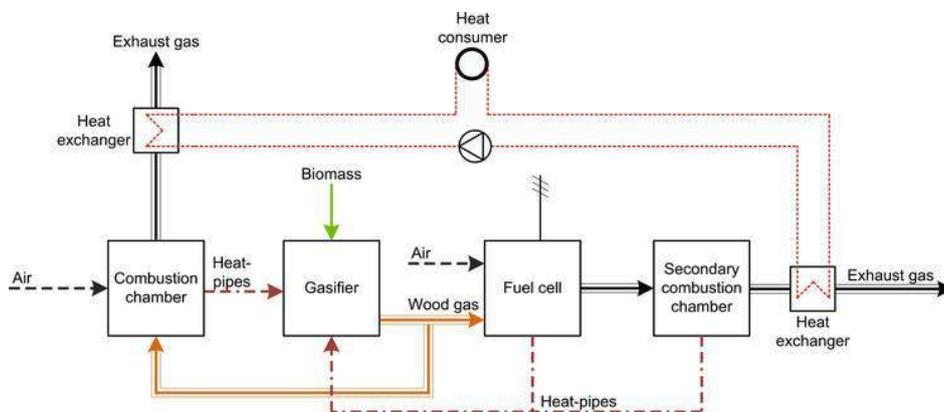
Figure 68: System diagram for a biomass CHP unit with fuel cell [29]
