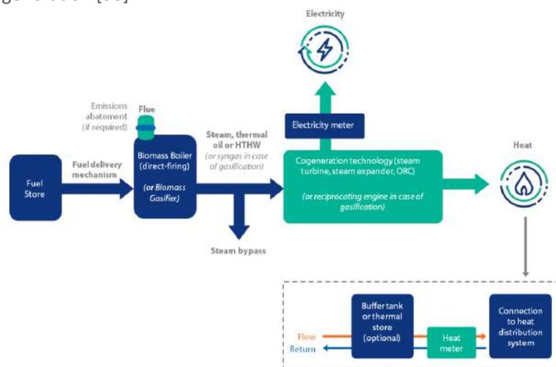
Figure 12: Typical biomass CHP components [38].
