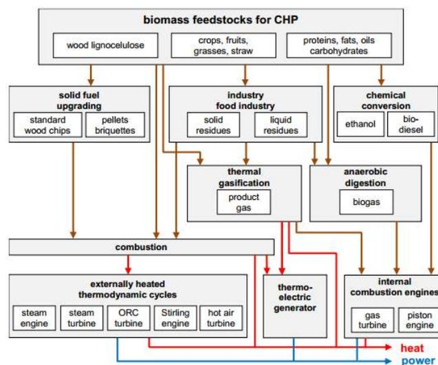
Figure 56: Most relevant paths of biomass feedstocks for CHP [9]
