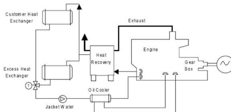
Figure 67: Closed-Loop Heat Recovery System for a Reciprocating IC Engine [27]
