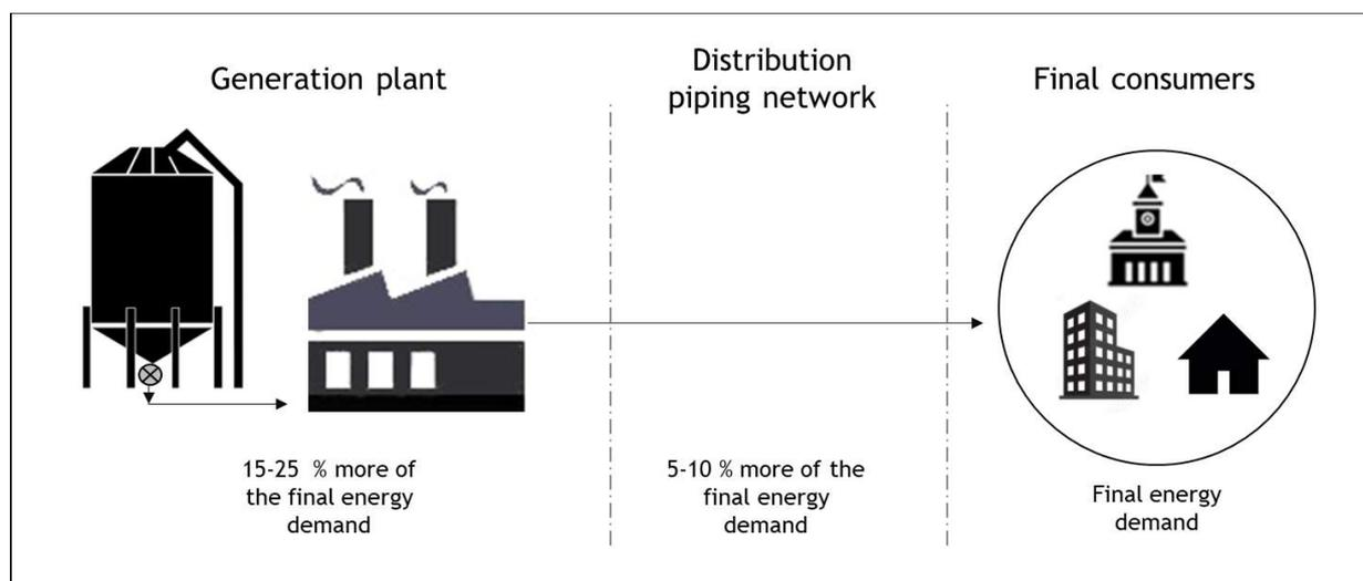
Figure 48. Basic scheme of the energy to be supplied in each part of the district heating system.
