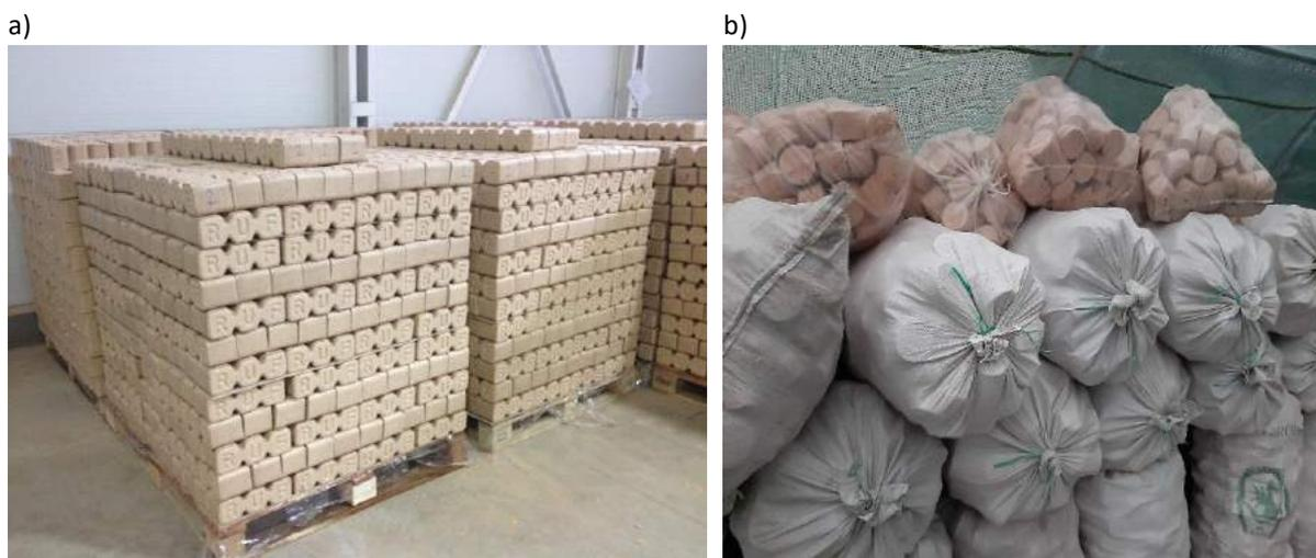
**Figure 37. Examples of storage options for briquettes [22], [23]:**
