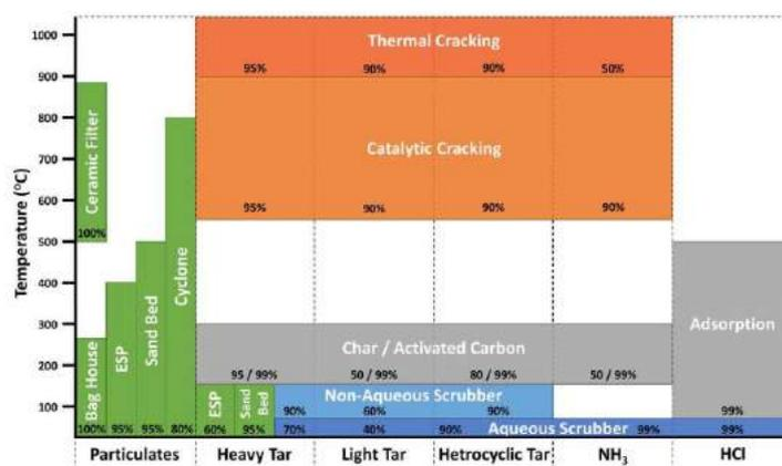
Figure 62: Syngas cleaning technologies including their applicable temperature range and efficiencies [23]
