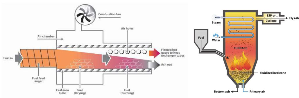
Figure 14. Fixed grate boiler (left) [42] and fluidized bed boiler (right) [43].
