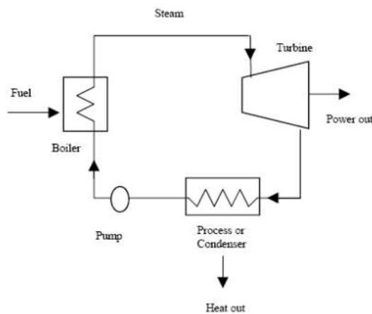
Figure 64: Steam turbine CHP system [27]
