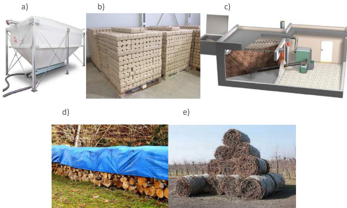
**Figure 4. Examples of fuel storage according to its size distribution. a) pellet storage in silo [12], b) briquettes storage in foiled pallets inside the room [13], c) woodchips storage [14], d) wood logs [15], e) bales storing outside logs [16].**
