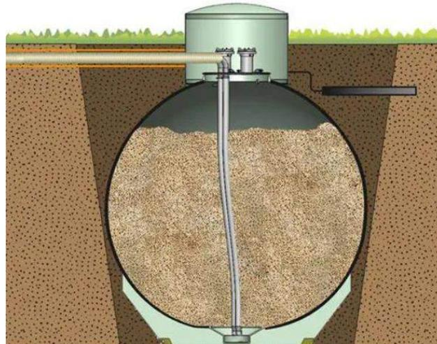
**Figure 34. Underground pellet storage silo [16].**
