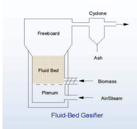
Figure 61: Fluidized-bed gasification systems [17]
