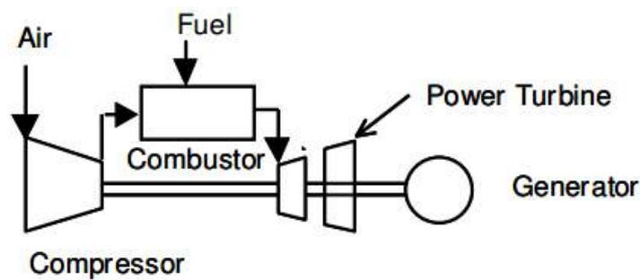
Figure 65: Components of simple-cycle gas turbine [28]
