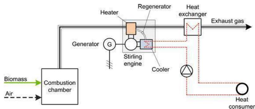
Figure 69: System diagram for a biomass CHP unit with a Stirling engine [32]
