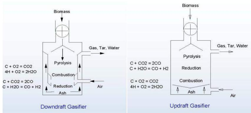
Figure 60: Fixed-bed gasification systems [17]
