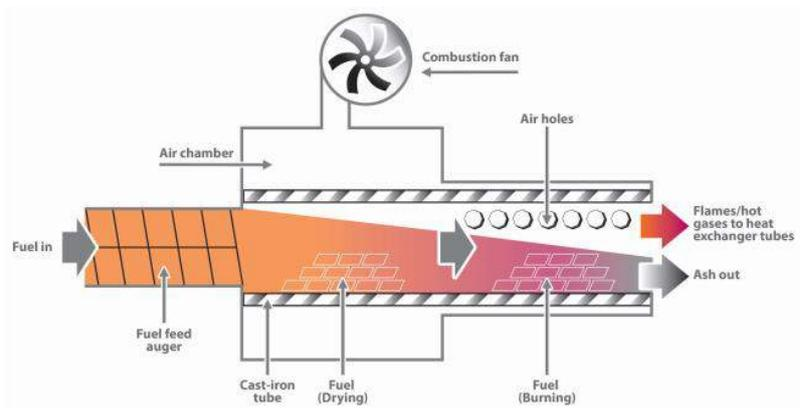
Figure 57: Fixed grate boiler [13]
