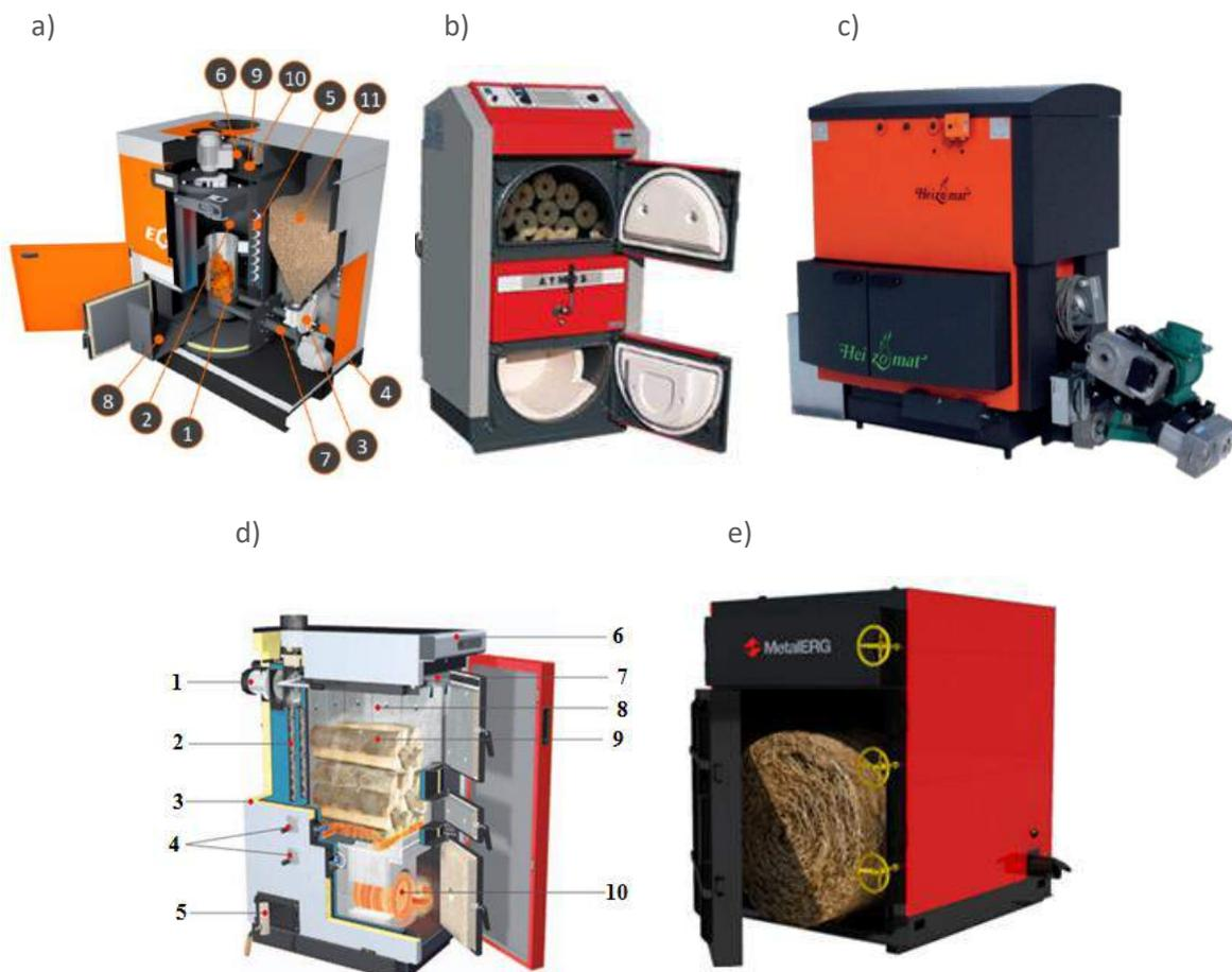
Figure 3. Different technology of biomass boiler according to the form of the biomass resource to be fed. a) pellet boiler [6], b) briquette boiler [7], c) Wood Chip Boiler [8], d) wood logs fired boiler [9], e) straw bales fired boiler [10].
