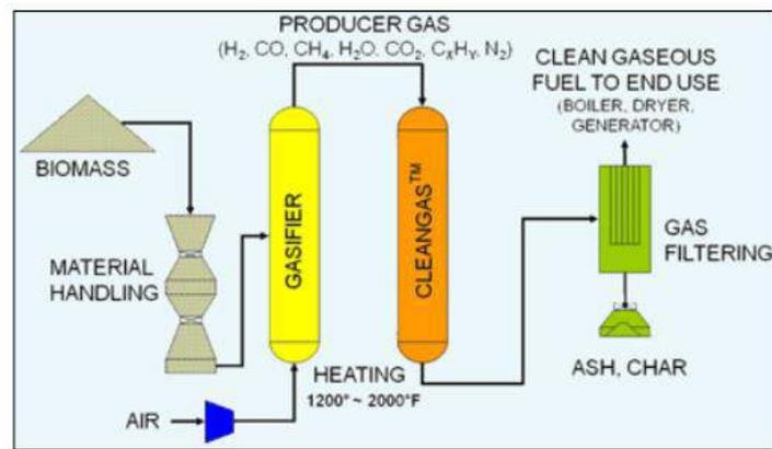
Figure 15: Example of two-stage gasification [44].
