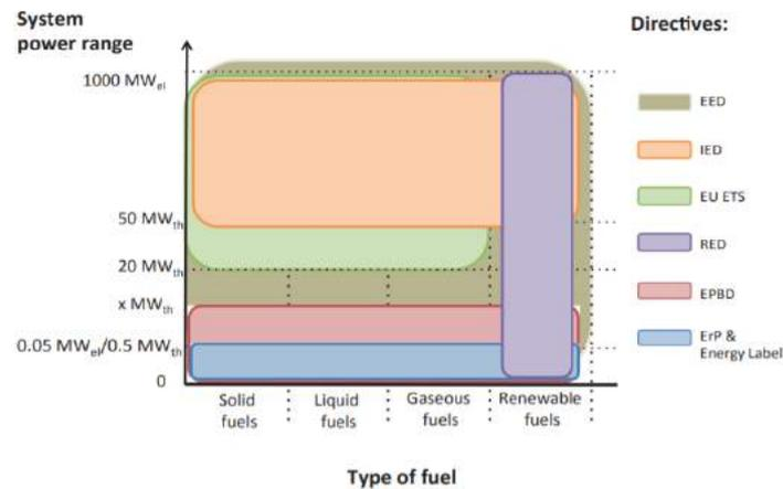
Figure 18. EU policies relevant for CHP based on fuel type and nominal power range [60].
