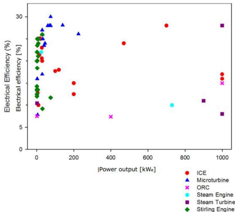
Figure 70: Electrical efficiencies of biomass conversion technologies based on power output [15]
