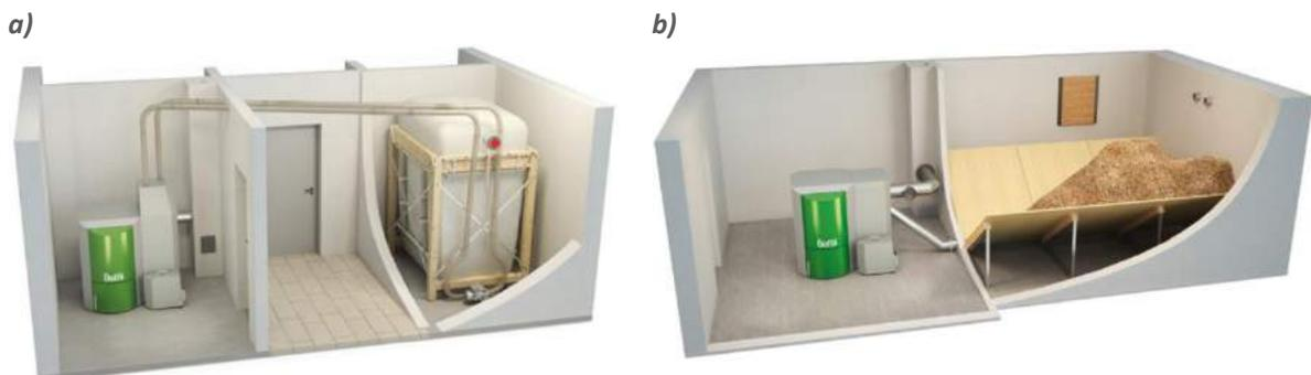
Figure 36. Examples of connecting a pellet boiler with a storage system [19].
