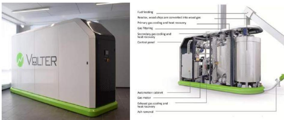
Figure 19. The CHP unit by Volter Oy fits, Volter 40 CHP Indoor [65].
