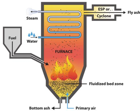
Figure 58: Fluidized bed boiler [14]
