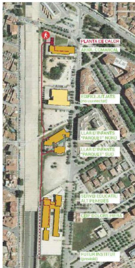
*Figure 51: Scheme of the District Heating in Vilafranca del Penedés.*
