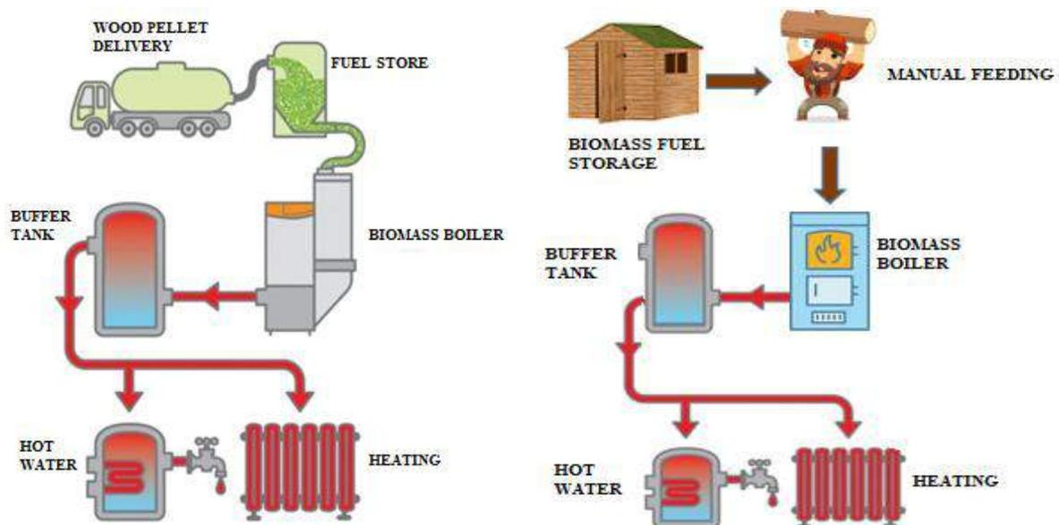
Figure 26. Main components of typical biomass direct heating installations [4]: a) automatic system of direct heating; b) manual system of direct heating.
