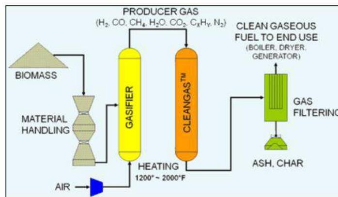
Figure 59: Example of two-stage gasification [16]
