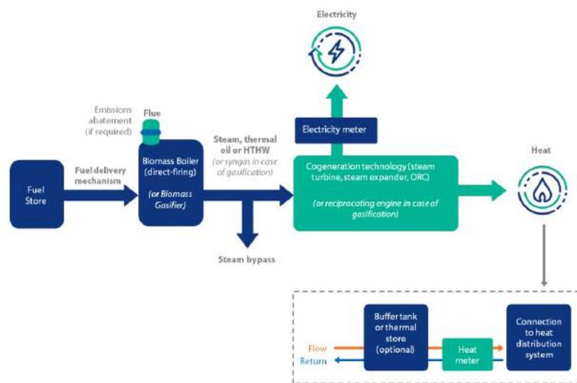
Figure 53: Typical biomass CHP components [1]
