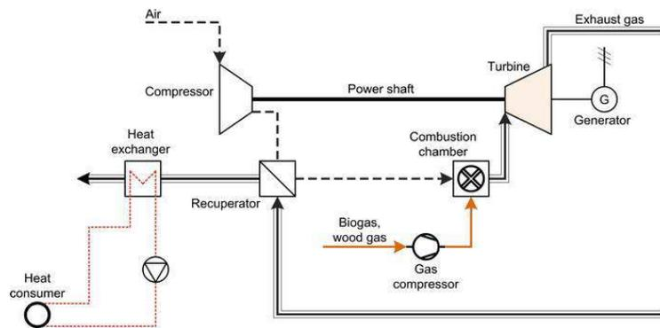
Figure 66: Microturbine-Based CHP System [30]
