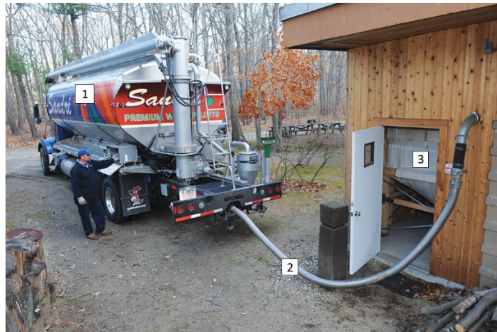
Figure 8. Pellets delivery process with the use of a tanker [33]: 1 – tanker, 2 – delivery pipe, 3 – prefabricated silos.
