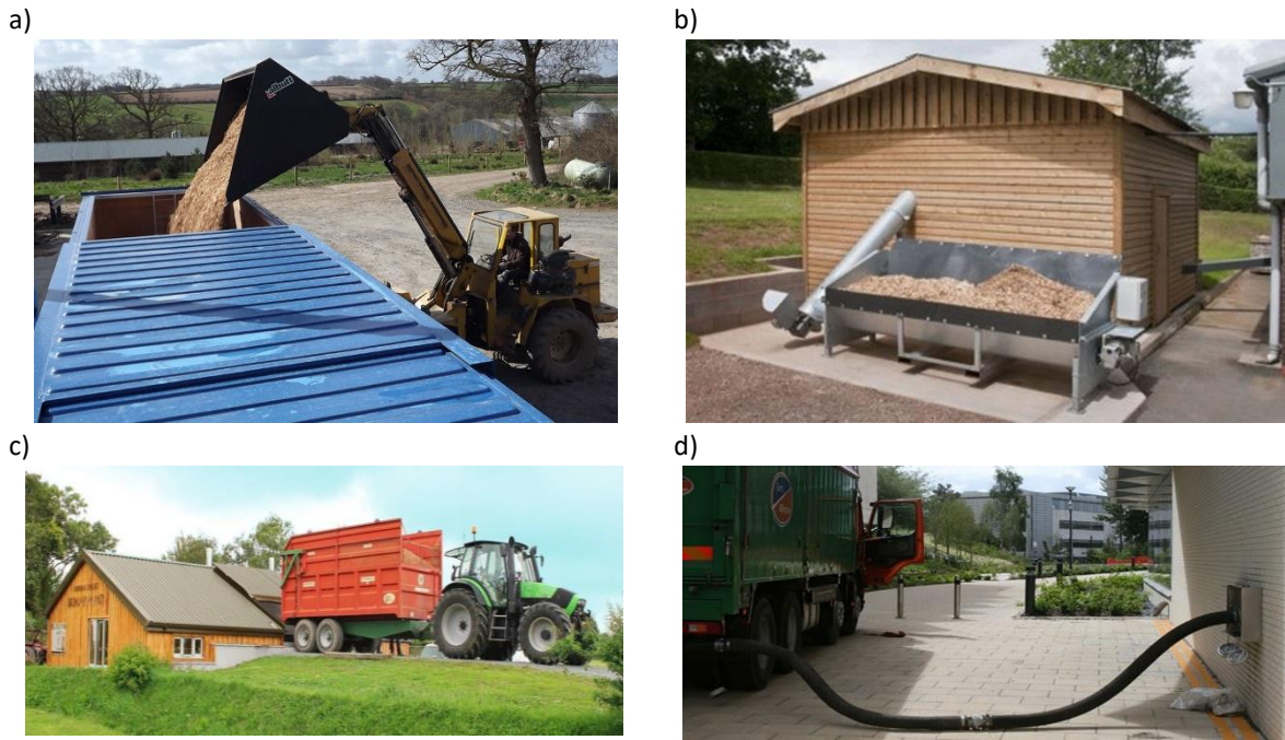
Figure 14. Chips deliver options, depending on storage scenarios [46]: a) tipped delivery into a bulk fuel store with tele handler chips moving; b) fast feed auger delivery; c) ramped delivery; d) blown delivery.
